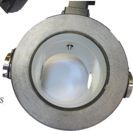
Clean White Glass Lined Internals of Valmet TS
